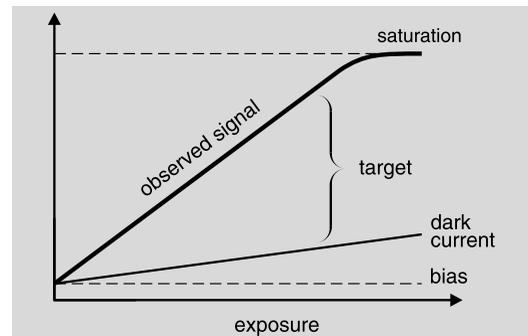
**Fig. 3.26** The signal measured by a CCD-camera depends almost linearly on the number of photons. During the exposure also the dark current will increase and has to be subtracted from the observed values. Bias is the dark current registered even if the exposure time were zero
