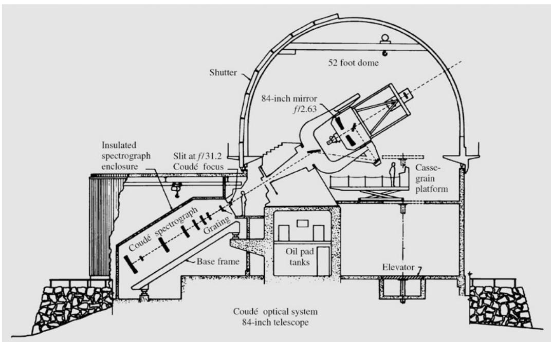
**Fig. 3.14** The coudé system of the Kitt Peak 2.1 m reflector. (Drawing National Optical Astronomy Observatories, Kitt Peak National Observatory)
