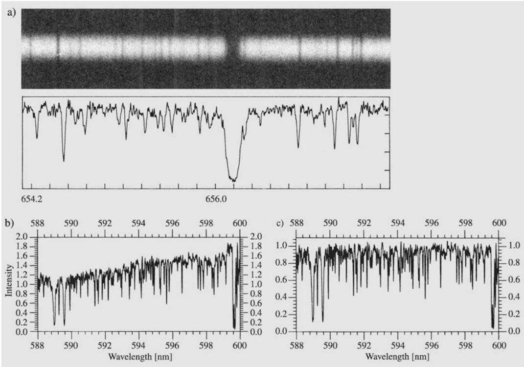
**Fig. 9.2** (a) A section of a photograph of a stellar spectrum and the corresponding rectified microdensitometer intensity tracing. The original spectrum was taken at the Crimean Observatory. (b) A more extensive part of the
