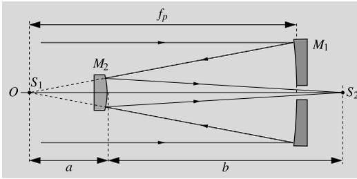
**Fig. 3.13** The principle of a Cassegrain reflector. A concave (paraboloid) primary mirror  $M_1$  reflects the light rays parallel to the main axis towards the primary focus  $S_1$ . A convex secondary mirror  $M_2$  (hyperboloid) reflects the rays back through a small hole at the centre of the main mirror to the secondary focus  $S_2$  outside the telescope
