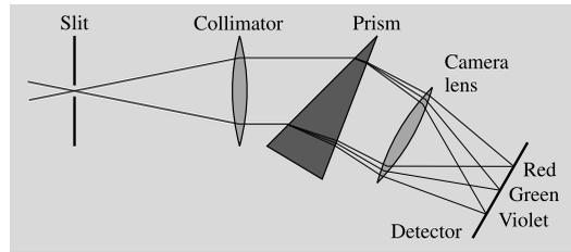
**Fig. 3.28** The principle of the slit spectrograph. Light rays entering through a slit are collimated (made parallel to each other), dispersed into a spectrum by a prism and projected onto a photographic plate or a CCD. There can also be several prisms. However, grids are used more commonly since they give a better resolution
