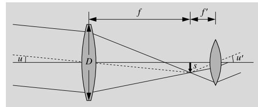
**Fig. 3.6** The scale and magnification of a refractor. The object subtends an angle  $u$ . The objective forms an image of the object in the focal plane. When the image is viewed through the eyepiece, it is seen at an angle  $u'$
