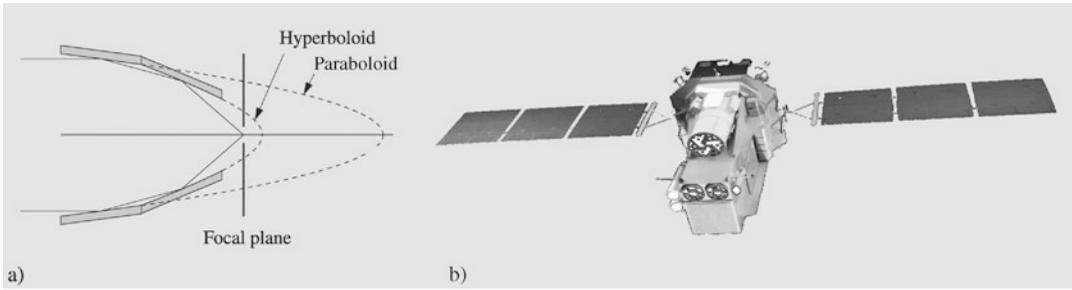
**Fig. 3.36** X-rays are not reflected by an ordinary mirror, and the principle of grazing reflection must be used for collecting them. Radiation meets the paraboloid mirror at a very small angle, is reflected onto a hyperboloid mirror
