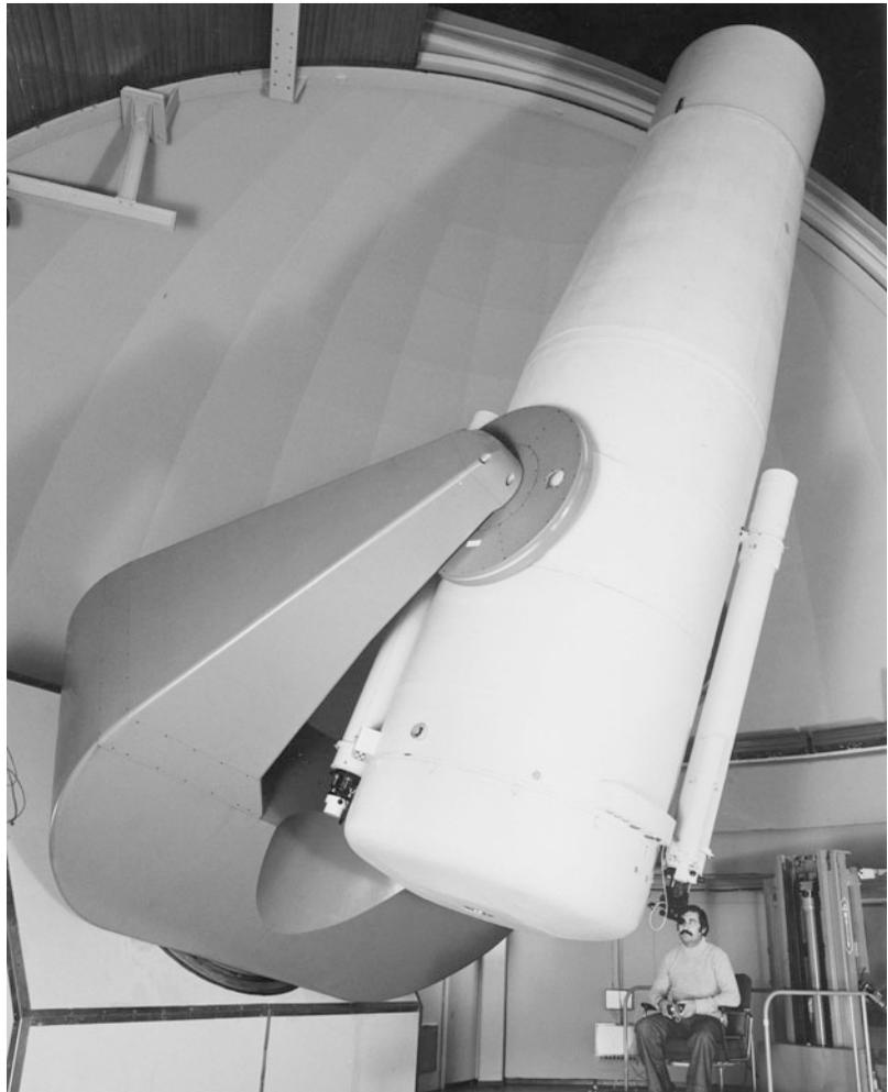
ward, the bearings must take an increasing load parallel with the declination axis.
