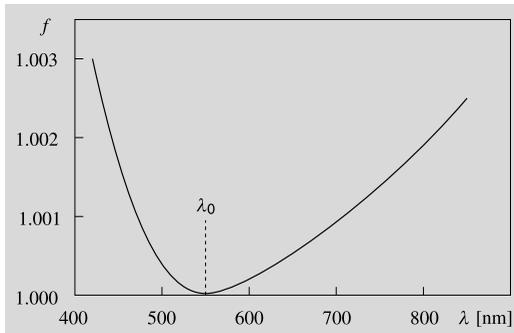
**Fig. 3.10** The wavelength dependence of the focal length of a typical achromatic objective for visual observations. The focal length has a minimum near  $\lambda = 550$  nm, where the eye is most sensitive. In bluer light ( $\lambda = 450$  nm) or in redder light ( $\lambda = 800$  nm), the focal length increases by a factor of about 1.002
