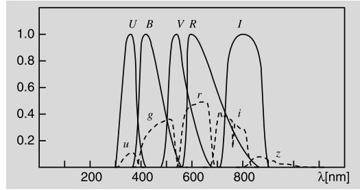
**Fig. 4.6** Relative transmission profiles of filters used in the UBVRI magnitude system. The maxima of the bands are normalised to unity. The R and I bands are based on the system of Johnson, Cousins and Glass, which includes also infrared bands J, H, K, L and M. Previously used R and I bands differ considerably from these. The curves of the *ugriz* magnitudes (*dashed lines*) give quantum efficiencies. They include the atmospheric extinction for airmass 1.3 (Sect. 4.5)
