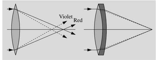
**Fig. 3.9** Chromatic aberration. Light rays of different colours are refracted to different focal points (*left*). The aberration can be corrected with an achromatic lens consisting of two parts (*right*)
