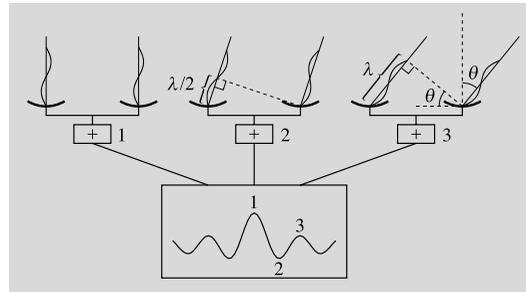
**Fig. 3.32** The principle of an interferometer. If the radiation reaches the radio telescopes in the same phase, the waves amplify each other and a maximum is obtained in the combined radiation (cases 1 and 3). If the incoming waves are in opposite phase, they cancel each other (case 2)
