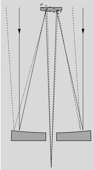
**Fig. 3.38** Refractors are not suitable for infrared telescopes, because infrared radiation cannot penetrate glass. The Cassegrain reflectors intended especially for infrared observations have secondary mirrors nodding rapidly back and forth between the object and the background near the object. By subtracting the brightness of the background from the brightness of the object, the background can be eliminated
