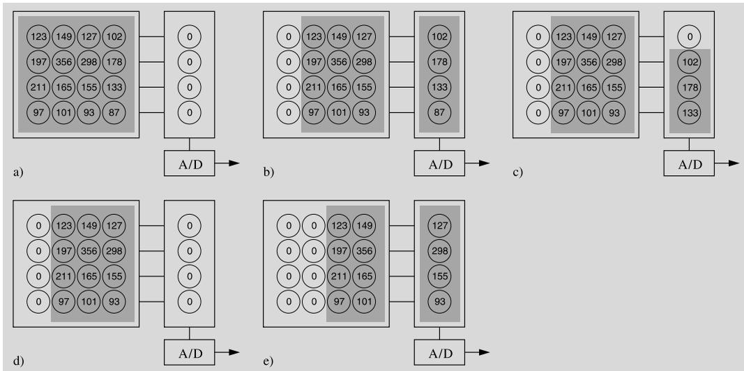
**Fig. 3.25** The principle of reading a CCD camera. (a) During an exposure electrons are trapped in potential wells corresponding to pixels of the camera. The number at each pixel shows the number of electrons. (b) After the exposure each horizontal line is moved one pixel to the right; the rightmost row moves to the readout buffer. (c) The contents of the buffer is moved down by one pixel.
